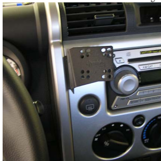
InDash installed showing Left side location.
