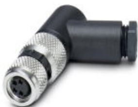
Connector, Universal, 4-position, Socket angled M8, A-coded, Screw connection, knurl material: Nickel-plated brass, external cable diameter 3.5 mm ... 5 mm
