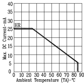
Fig5. MAX. ALLOWABLE DC CURRENT VS. AMBIENT TEMPERATURE.
