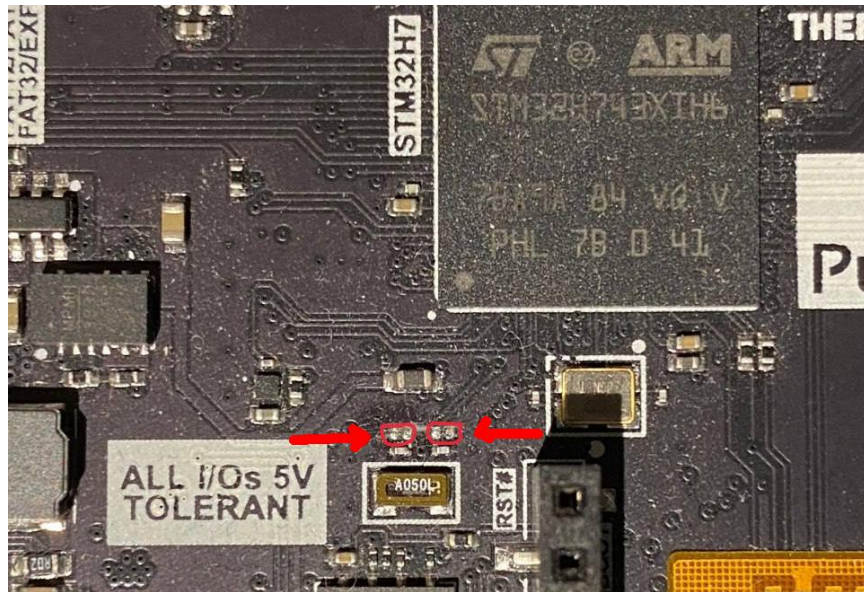
Figure 4: C96 and C97 are located adjacent to the STM32 package as shown.
