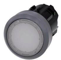
Illuminated pushbutton, 22 mm, round, plastic with metal front ring, white, pushbutton, flat, latching, Push-to-release mechanism, with laser labeling, symbol number according to, ISO 7000 or IEC 60417
