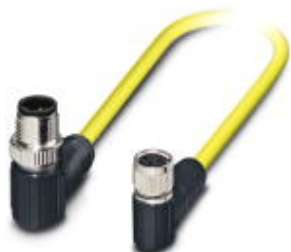
Sensor/actuator cable, 3-position, PVC, yellow, shielded, Plug angled M12 SPEEDCON, A-coded, on Socket angled M8, cable length: 1.5 m
