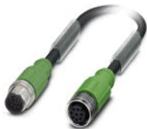
Sensor/actuator cable, 8-position, Variable cable type, shielded, Plug straight M12, A-coded, on Socket straight M12, A-coded, cable length: Free input (0.2 ... 40.0 m)
