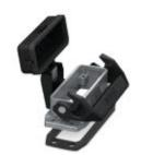
Panel mounting base D25, with single locking latch, material: Die-cast aluminum, salt water resistant, protective cover material: PA, height: 26 mm, cable gland: none, support sleeve: no, protective cover: yes, Standard
