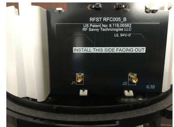
Fig 1.0 AMC-RFCRFS005B-A RF Coupler Installed in kV2C Meter
