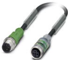
Sensor/actuator cable, 3-position, Variable cable type, Plug straight M12, A-coded, on Socket straight M12, A-coded, with 2 LEDs, cable length: Free input (0.2 ... 40.0 m)
