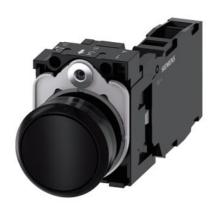
Pushbutton, 22 mm, round, plastic, black, pushbutton, flat, momentary contact type, with holder 1 NO+1 NC, screw terminal, with laser labeling, inscription or symbol Customer-specific selection with SIRIUS ACT configurator (CIN)
