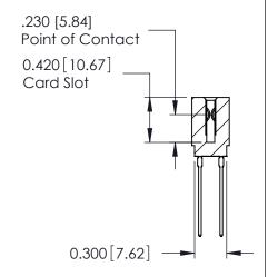
ACAD REFERENCE NO. 725-ENG MASTER 725 Series Ultra-Mate Card Edge Connector - Press Fit DRAWN: J.LEE DATE: AUG31/09 Part Number: 725-014-541-201 SEGTION A-A CHECKED: SHEET 1 OF 1 **EDAC INC** SCALE: THESE DRAWINGS AND SPECIFICATIONS ARE THE PROPERTY OF EDAC INC.,AND TORONTO, ONTARIO SHALL NOT BE REPRODUCED, OR COPIED DRAWING NUMBER **ISSUE** CANADA OR USED AS THE BASIS FOR THE 725-ENG MASTER MANUFACTURE OR SALE OF APPARATUS YOUR CONNECTION TO QUALITY & SERVICE WITHOUT WRITTEN PERMISSION.
