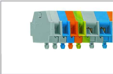
Terminal strip with snap-in mounting feet, for 0.6 ... 1.2 mm plate thickness, 3.5 mm mounting hole diameter (also for 210-154 Aluminum Rail or with 209-120 Mounting Foot for DIN-35 rail)
