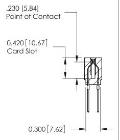
ACAD REFERENCE NO. 725 Series Ultra-Mate Card Edge Connector - Press Fit DRAWN: Part Number: 725-052-545-201 CHECKED: SCALE: **EDAC INC** THESE DRAWINGS AND SPECIFICATIONS ARE THE PROPERTY OF EDAC INC., AND TORONTO, ONTARIO SHALL NOT BE REPRODUCED, OR COPIED
