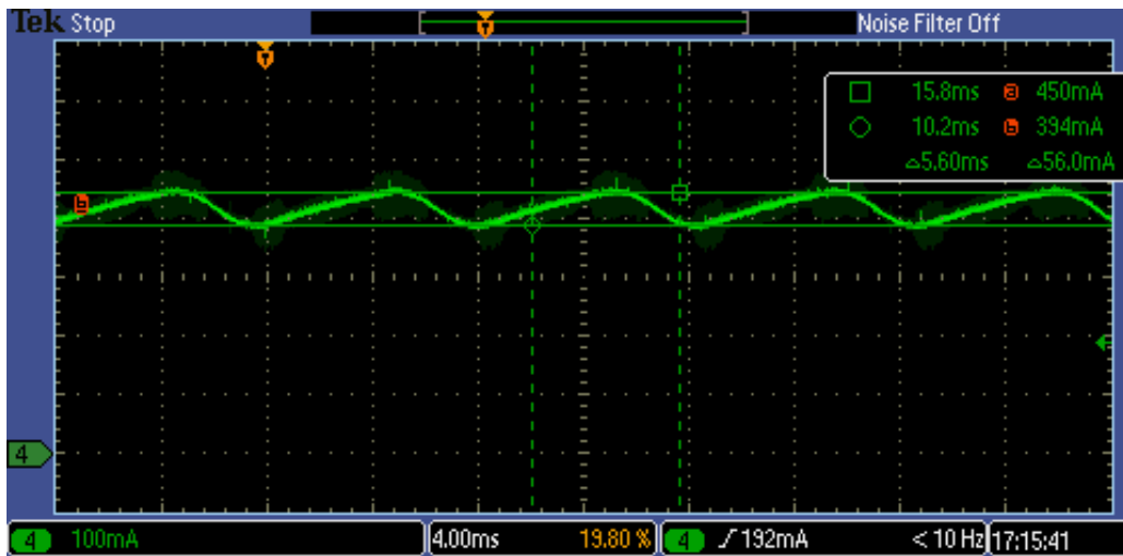
Figure 14. Output Ripple 13% Pk - Pk
