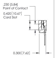
725 Series Ultra-Mate Card Edge Connector - Press Fit Part Number: 725-019-540-101
