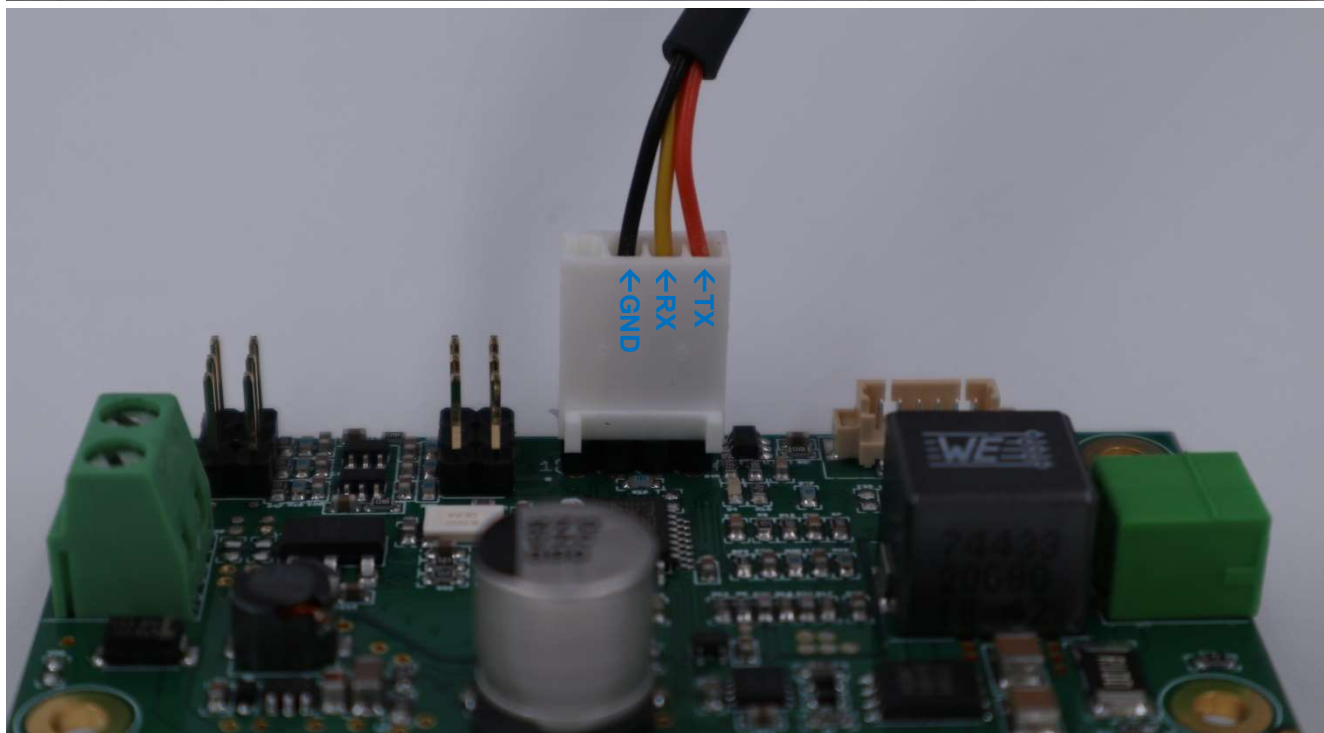
Figure 17: Drive F connection to the USB-TTL-Converter
