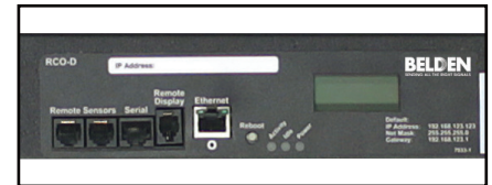
Intelligent PDU Communication and Environmental Monitoring Ports
