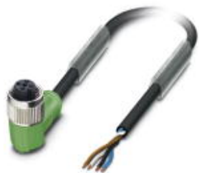
Sensor/actuator cable, 4-position, PUR halogen-free, black-gray RAL 7021, free cable end, on Socket angled M12, A-coded, cable length: 25 m
