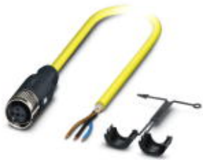
Sensor/actuator cable, 3-position, PVC, yellow, shielded, free cable end, on Socket straight M12 SPEEDCON, A-coded, cable length: 2 m
