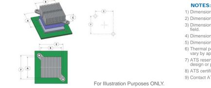
1) Dimension A is the length of the heat sink in the direction of the flow.
