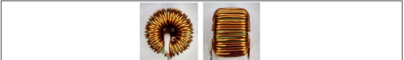
Figure 7 Photos of the PFC choke
