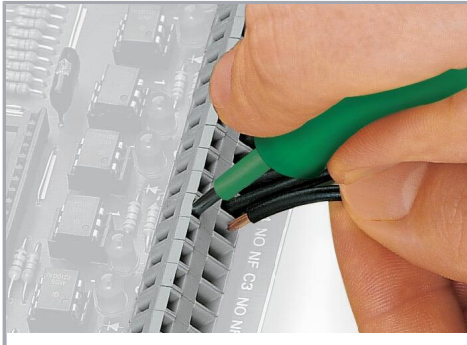
Inserting a conductor via 3.5 mm screwdriver.
