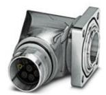
Device connector, front mounting, angled rotatable, for standard and SPEEDCON interlock, M17, number of positions: 7+PE, type of contact: Pin, Crimp connection, Axial O-ring, 4x Ø 3.2, shielded: yes, flange dimensions: 25.75 mm x 25.75 mm
