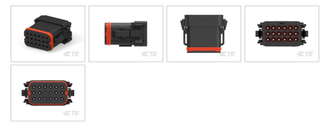
Connector & Housing Type: Housing for Female Terminals Mating Pin Diameter: 1.59 mm [.063 in ] Connector System: Wire-to-Wire
