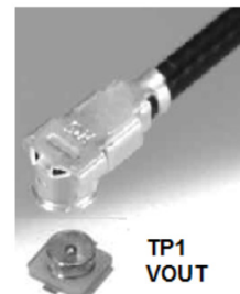
Figure 3. Technique for Measuring Output Ripple and Step Response with a Low Inductance Connector (Not Supplied)
