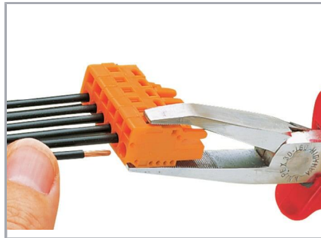
Inserting a conductor via operating tool.
