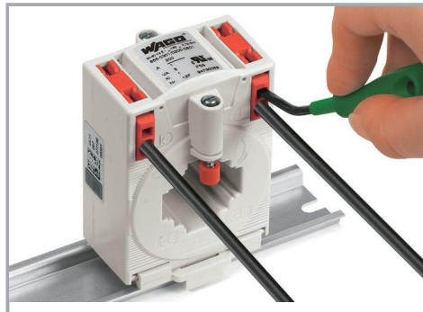
Conductor termination – screwdriver actuation parallel to conductor entry
