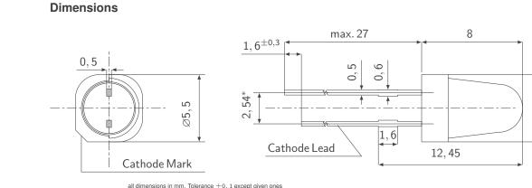
all dimensions in mm. Tolerance  $\pm 0,\,1$  except given ones at the bottom of the LED
