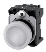
Indicator lights, 22 mm, round, metal, shiny, white, lens, smooth, with holder, LED module with integrated LED 24 V AC/DC, screw terminal, with laser labeling, upper case
