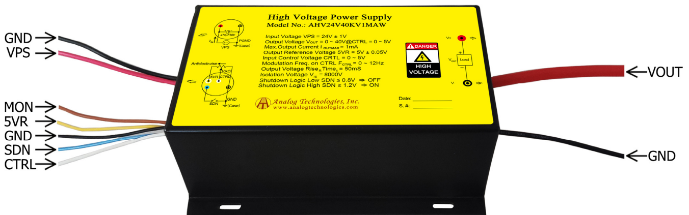
Figure 2. The Connecting Lead Wires of AHV24V40KV1MAW
