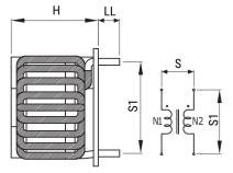
**General Information** Series SC-JH Style Through-Hole RoHS Yes Lead Spacing (S/S1) Are For Reference Only. Notes Miscellaneous Temperature Rise Maximum: 50 K. Core Mn-Zn Ferrite
