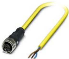
Sensor/actuator cable, 3-position, PVC, yellow, free cable end, on Socket straight M12 SPEEDCON, A-coded, cable length: 10 m
