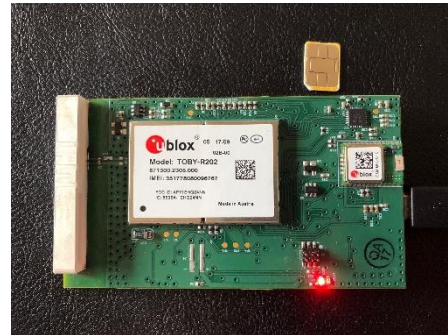
LED Blinking RED after Failed Test
