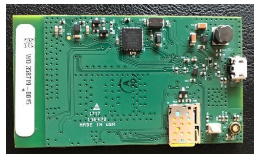
SIM Entirely Inserted and Locked
