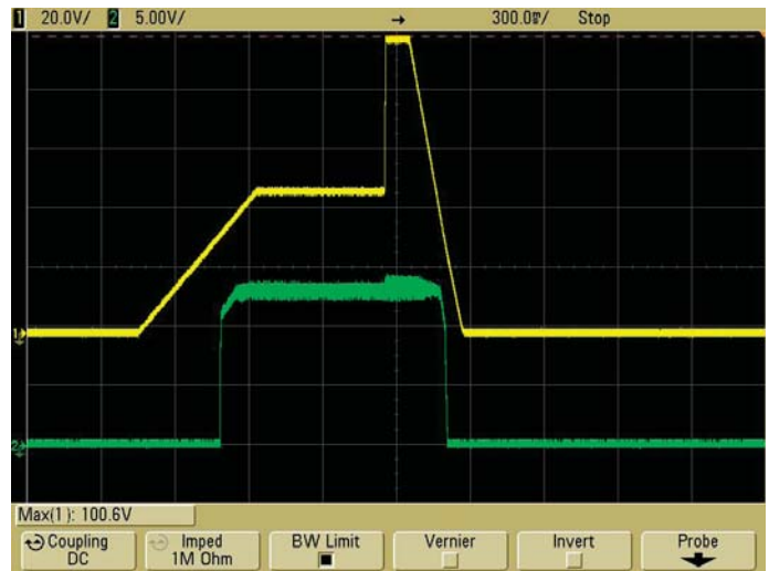
Figure 4. Test Waveform with Feedback Loop Open
