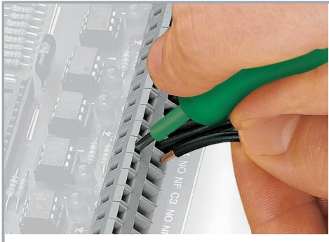
Inserting a conductor via 3.5 mm screwdriver.
