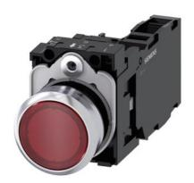
Illuminated pushbutton, 22 mm, round, metal, shiny, red, pushbutton, flat, momentary contact type, with holder, 1 NO+1 NC, LED module with integrated LED 24 V AC/DC, screw terminal, Z=20-unit packaging
