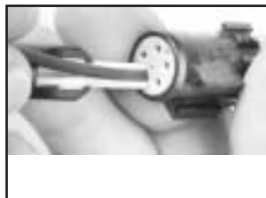
2. Using a straight motion forward, insert the tool along the wire until it bottoms against the connector. (Do not use a screwing motion - damage will result.)
