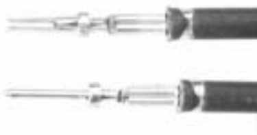
8. Note that there are no unterminated wire strands, and that some strand ends can be seen at the forward edge of the crimp. Also note the insulation is gripped by the smaller secondary crimp. Distortion is at a minimum, both axially and laterally - no sharp edges.
