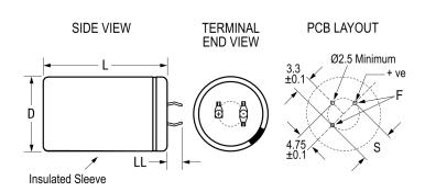
General Information Series ALC70 Dielectric Aluminum Electrolytic Description Snap-In, Aluminum Electrolytic RoHS Lead 3 Pin Short AEC-Q200 No Halogen Free Yes Component Weight 60 g Notes Dimensions D And L Include Sleeving. Shelf Life 156 Weeks
