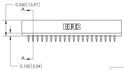
0.420 [10.67] Card Slot 0.34 [8.53] 0.31 7.77 Point of Contact 0.550 13.97 0.300 [7.62] SECTION A-A
