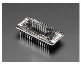
Populating the **8x2** row header at the center of the board (16 pins total) provides a "Fadecandy-style" connection.
