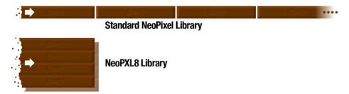
\* Hypothetical situation, not an imposed limit. Depends on available RAM, but most "M0" (SAMD21) boards might handle upwards of 2,500 pixels, with "M4" (SAMD51) potentially up to 15,000...but in reality, you'll want some *fraction* of that, so your code has time to *compute* those pixels.
