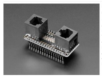
Populating the two RJ45 connectors at the board ends provides an "OctoWS2011-style" connection.
