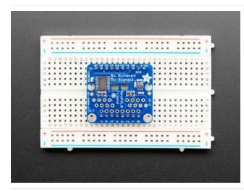
A third option is to install header pins on the NeoPixel outputs, so both the "ins" and "outs" are breadboardable...this may be useful for certain prototyping tasks.
