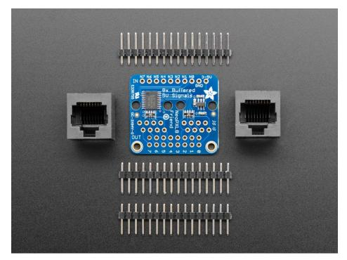
If you're working on a solderless breadboard or aren't using a Feather form-factor microcontroller, the Adafruit NeoPXL8 Friend (https://adafru.it/CJd) provides similar utility to the NeoPXL8 FeatherWing but in a non-FeatherWing package.
