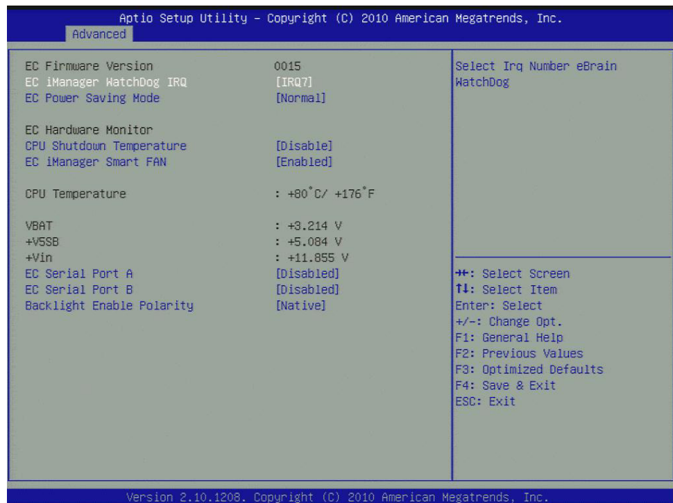
Figure 3.12 Embedded Controller Configuration
