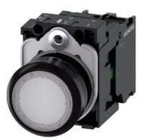
Illuminated pushbutton, 22 mm, round, plastic, white, pushbutton, flat, momentary contact type, with holder, 1NO, LED module with integrated LED 24 V AC/DC, screw terminal, with laser labeling, symbol number according to, ISO 7000 or IEC 60417
