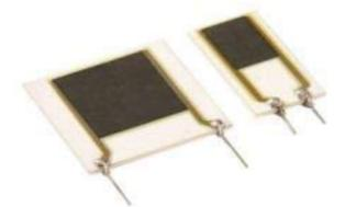
A range of non-inductive thick film power resistors complementing the T0220 packaged MPT series (20 Watt heat sink styles), being vertically mounted and suitable to dissipate power from 3 Watts up to 10 Watts. Available in values from 1R0 to 200K ohms they are the ideal solution for small snubber circuits, the output side of high speed pulse generators and low inductive resistor requirements in switch mode power supplies.
