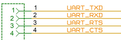
Figure 15: Bluetooth over UART interface
