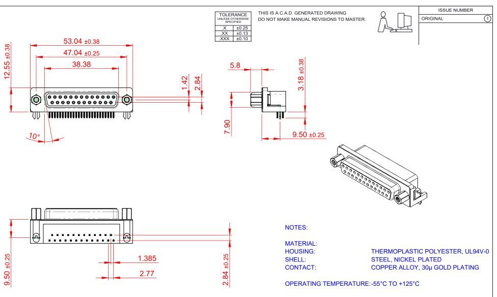
**CURRENT RATING: 3A PER CONTACT** CONTACT RESISTANCE: 25mΩ MAX. **INSULATOR RESISTANCE:** 5000MΩ min. DIELECTRIC WITHSTANDING VOLTAGE: 1000V AC rms
