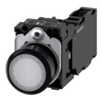
Illuminated pushbutton, 22 mm, round, plastic, white, pushbutton, flat, momentary contact type, with holder, 1 NO+1 NC, LED module with integrated LED 24 V AC/DC, screw terminal, with laser labeling, symbol number according to, ISO 7000 or IEC 60417
