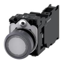
Illuminated pushbutton, 22 mm, round, plastic with metal front ring, clear, pushbutton, flat, momentary contact type, with holder, 1 NO+1 NC, LED module with integrated LED 24 V AC/DC, spring-type terminal, Z=20-unit packaging
