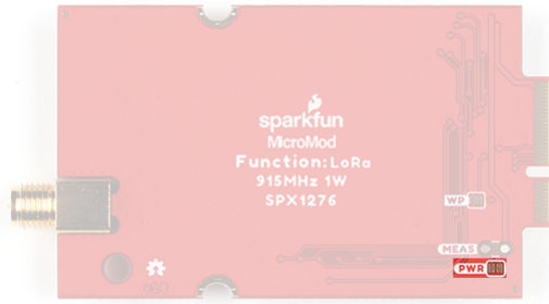
LED power jumper on the LoRa MicroMod Function Board. (Click to enlarge)
