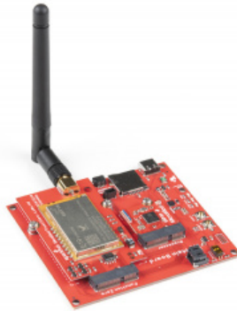
Fully assembled main board with processor board and function board. (Click to enlarge)
