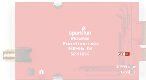
EEPROM WP jumper on the LoRa MicroMod Function Board. (Click to enlarge)
