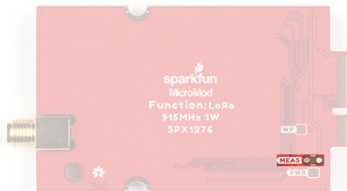
Current measurement jumper on the LoRa MicroMod Function Board. (Click to enlarge)
