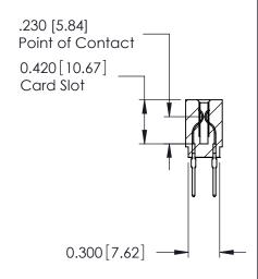
725 Series Ultra-Mate Card Edge Connector - Press Fit ACAD REFERENCE NOSECTION SARA
